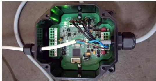
[Figure 5] Encoder and sensors signals secondary hub A1-RE1024
